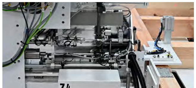
Screw unit for screwing frame works together.
