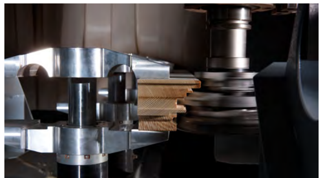
Liquid-cooled trimming spindles with vector control
