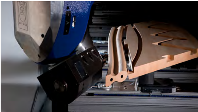
Paling holes at a tight angle
